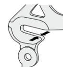
Cannot use fork thicknesses less than 6 mm.
