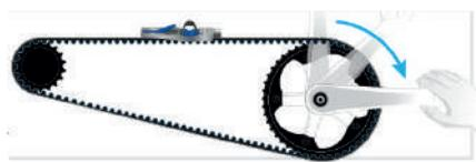
The average measured tension must be between 43lbs and 47lbs.
