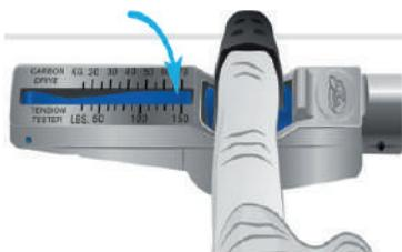
1. Check that the indicator arm is fully lowered. Place your index finger inside the rubber finger strap over the click pad as shown.
